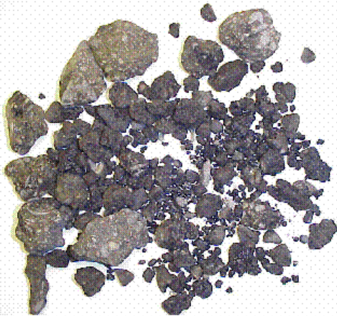
Figure 2.16: RAP in Aggregate-Sized Chunks
