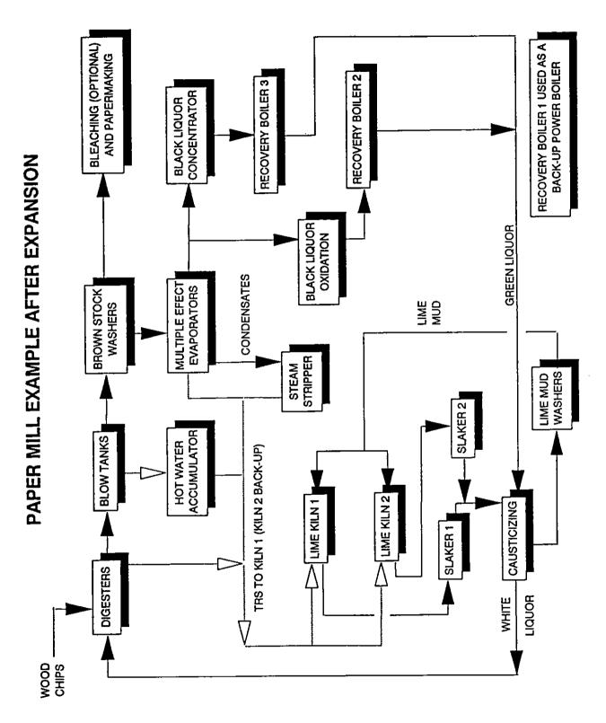
Figure 2. Paper mill flow diagram after proposed expansion.
