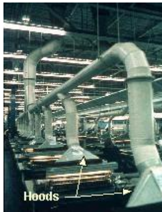
Figure 3-12. Stationary hood in an industrial process.
